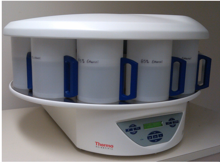
Figure 3.36: Thermo Scientific Spin Tissue Processor for dehydration, clearing, and infiltration of tissue for histology.
