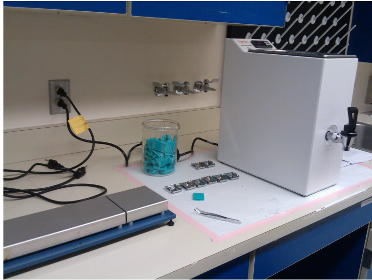
Figure 3.37: Tissue embedding station showing hot plate (left), tissue holder cassettes (center), and paraffin wax dispenser (right).
