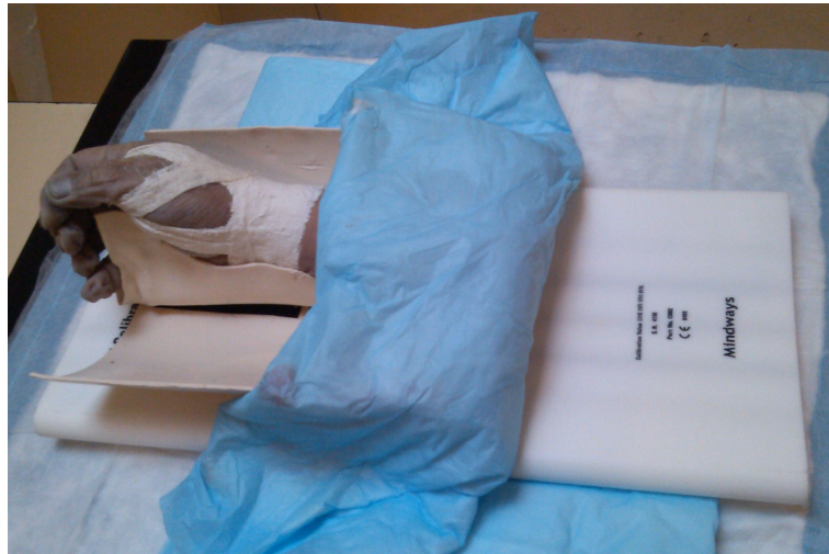
Figure 5.2: Cadaveric specimen (right hand) placed in a modified forearm splint attached to the top surface of a QCT calibration phantom for CT scanning.
